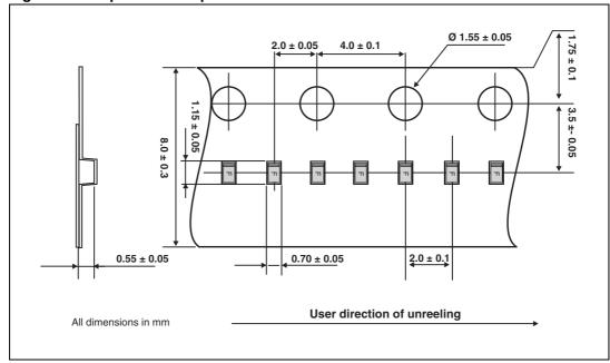
Figure 11. Tape and reel specification
